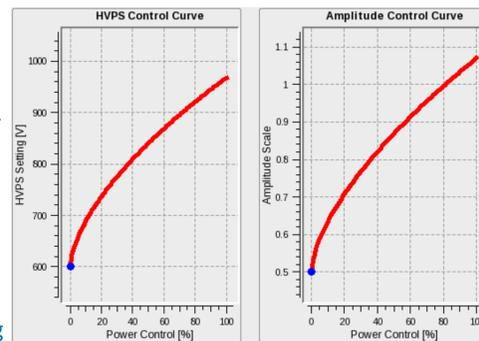
Figure 7: Feedforward control laws for klystron mod. and RF drive
