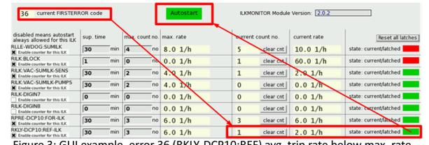
Figure 3: GUI example, error 36 (RKL-DP10:REF) avg. trip rate below max. rate
