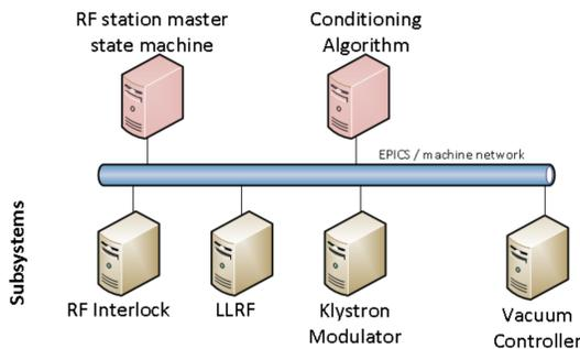
Figure 1: Subsystem setup, control system perspective
