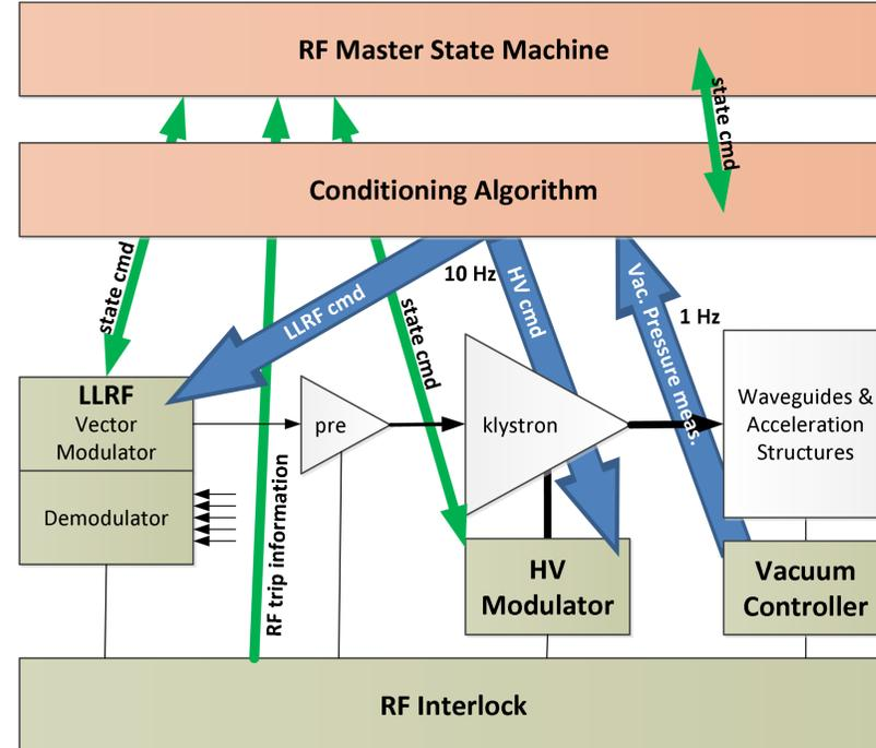
Figure 2: Single RF station subsystem setup, hierarchy and interactions
